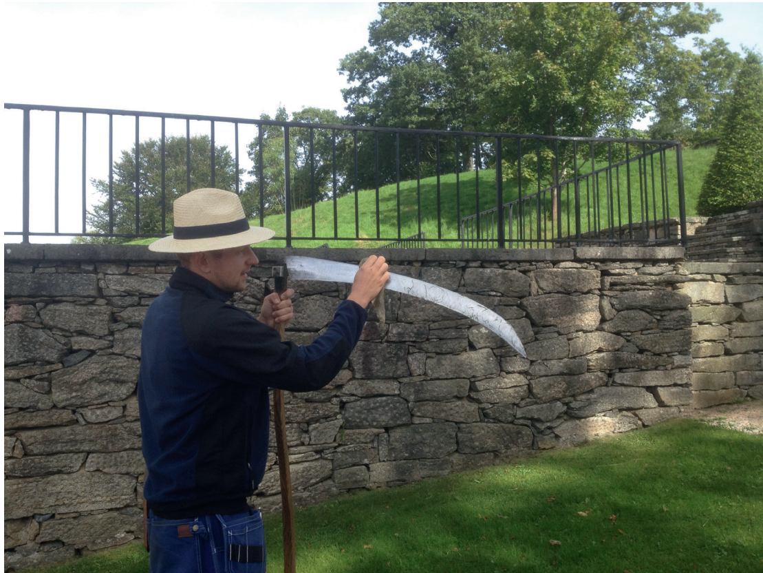
Figure 3: Cleaning the scythe blade with a textile cloth before sharpening with the whetstone—a practice-based solution to a problem that proved to be recommended by Abercrombie in the eighteenth century as well. Photograph by Daniel Lundberg 2012.
